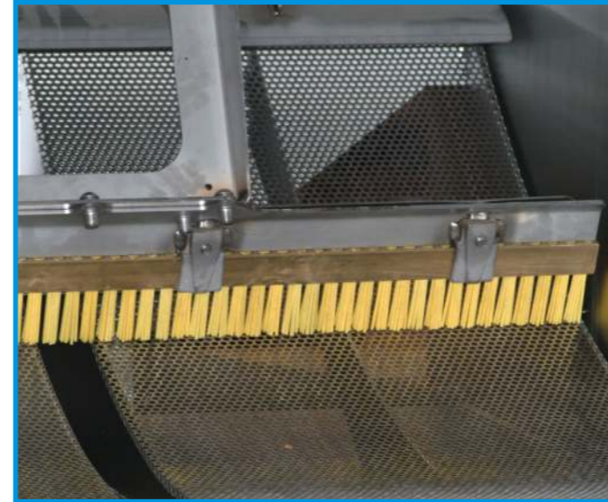
Brushed perforated screen with 3 or 6mm holes
